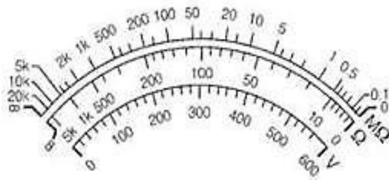
Fig.2. Typical scale on the Megger insulation tester .Factors affecting insulation resistance readings:
